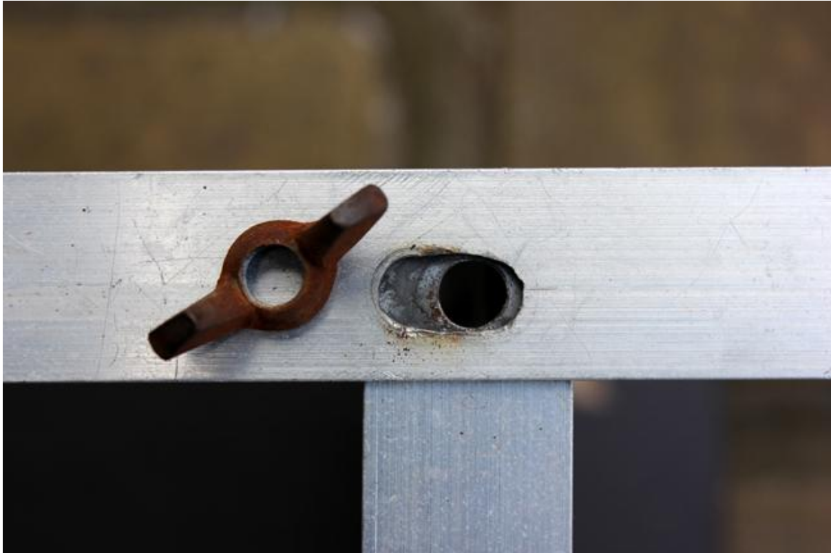
Figure 5. Slot in the L shaped lengths at the bottom of the box.
